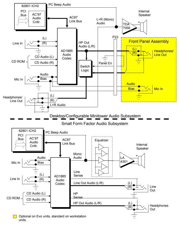
Figure 5-10. Audio Subsystem Functional Block Diagram
